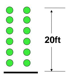
Cross Section of Individual Exchanger (liquid in annulus)
